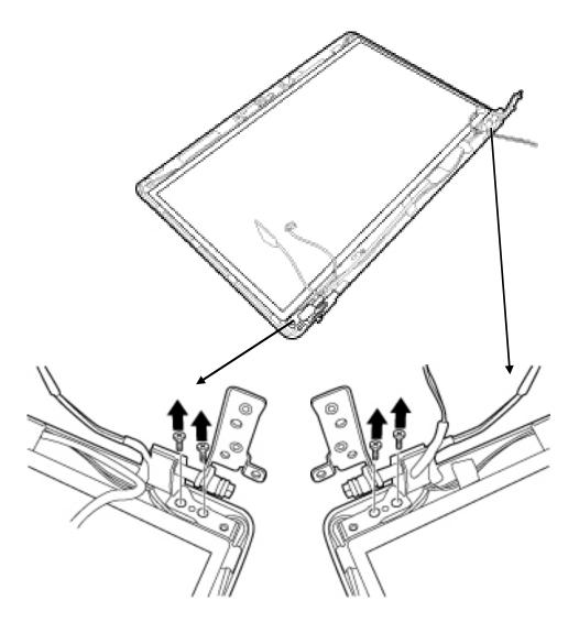
Figure 4-46 Removing the LCD unit
